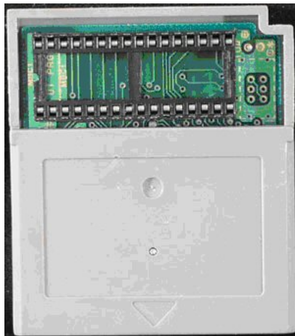
Figure 4. Cartridge for the Nintendo Game Boy with space for custom erasable programmable read-only memory (EPROM) chip (Handheld Museum, 2008).
